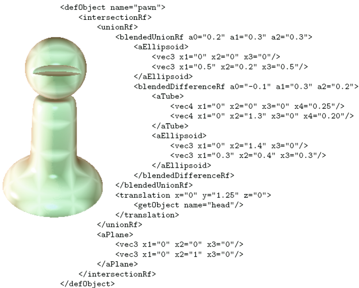
Fig. 4. A demonstration of the XISL language (script) that defines the implicit "pawn" object and the rendered image of the script
